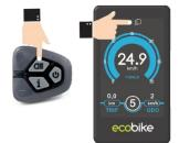
With the turned on display, click on / off at once the lights button to turn on the display backlight and the front and rear lights. Click the button again to turn off the backlight and lights. When the light is on, you can see the icon on the screen as in the picture beside.
