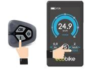
When the electrical system is turned on, the display will show the speed and distance as defaults.
