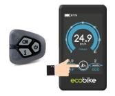
Press and hold the "MINUS" button to start the motor that will go at 6km / h without pedaling. The display will show the icon as in the picture beside. When the user releases the button, the engine will automatically shut down.
