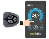
Indicates the power with which the motor works, when the entire power bar is displayed, this means that the motor works at full power. The battery is discharged faster then.
