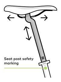
Adjust the seat post to the desired height and clamp it tightly. The seat pin should be inserted into the frame so that the safety marking on the pin is hidden. If you can see the marking, there is a risk of the seat pin breaking during the ride. Such an accident may also break the frame under the seat.
